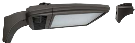
EES-KH45Q Shown with "KH45A" Kitty Hawk Arm, Kitty Hawk Die-Cast Mounting Arm, Bronze Powdercoat Finish, Includes Hardware. Mounts Directly to Square Poles. Replacement Model KH45AZ.
